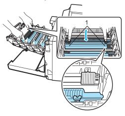
2 Clean the corona wire inside the drum unit by gently sliding the green tab from left to right and right to left several times.
